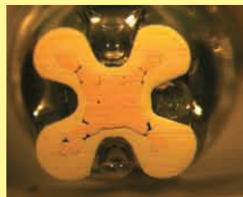
Crimp-cross section HARTING crimp profile
